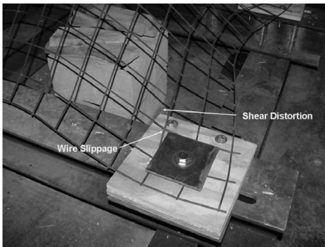
Figure 9. Shear distortion of wire squares and slippage of wire from under the plates.
